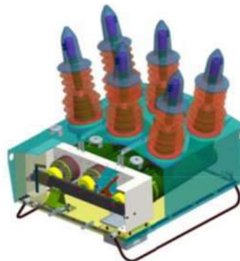
Figure 1 3D Modelling in Smart Recloser Design
