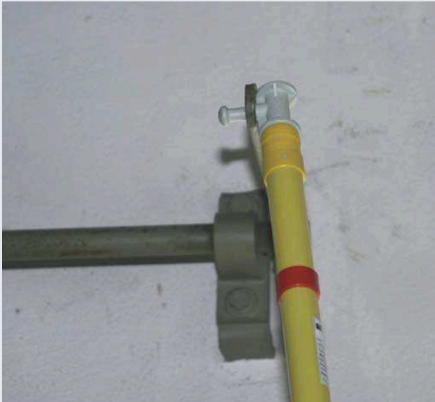
Switching stick head screwed on an IS SK insulating stick for switching a switch disconnector
