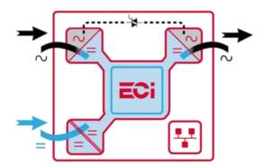
The ECI technology eliminates all single points of failure with full scalability; up to 32 modules in parallel and high efficiency of up to 96% in AC to AC conversion, and above 93.5% in DC/AC conversion, hence reducing operating costs. We can build the systems up to 2.7 MVA.
